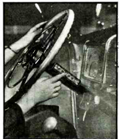
Fig. H. Stations are tuned-in by just pushing the 5 buttons on this steering-column unit.
