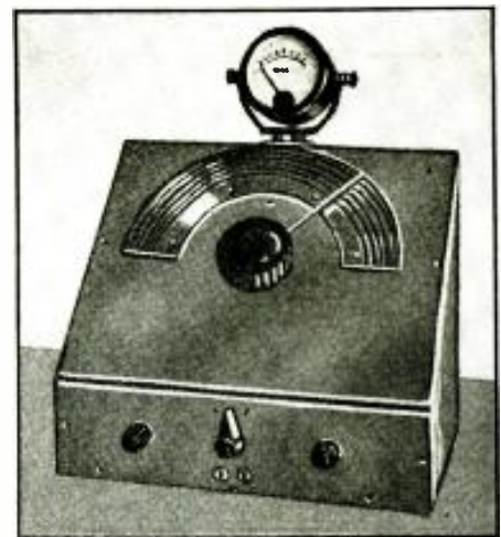
Fig. A. A new French bridge capacity meter.
