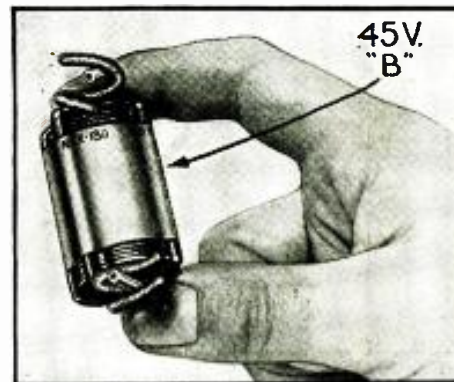
Fig. A. The appearance of the complete layerbuilt battery. The comparative size can be seen against the hand.
